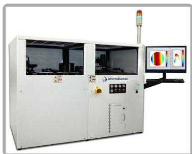
The MicroSense UltraMap C200A is an automated LED Sapphire Wafer Measurement system based on MicroSense's proprietary two sided capacitive sensing technology. The system measures critical substrate parameters including Thickness, TTV, Bow, ...
